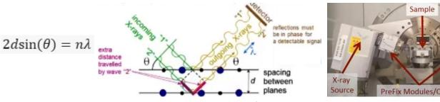
where d is the interplanar spacing,  $\theta$  is the Bragg angle, n is the reflection order, and  $\lambda$  is the wavelength of X-rays.
